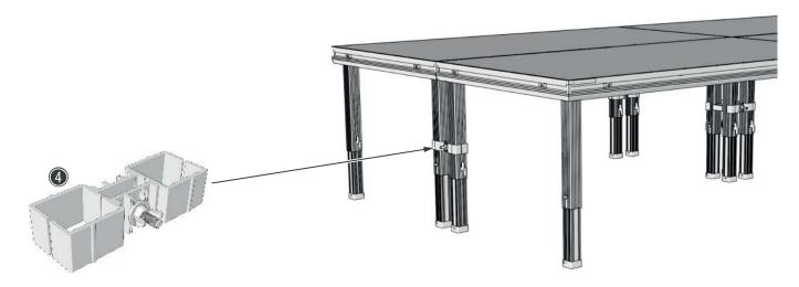
**3.** Fix two plug-in feet standing side by side with a dual plug-in feet connector (4) and tighten the wing screws.
