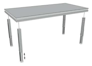
**1.** Insert the plug-in feet into the provided recess on the bottom of the stage platform.
