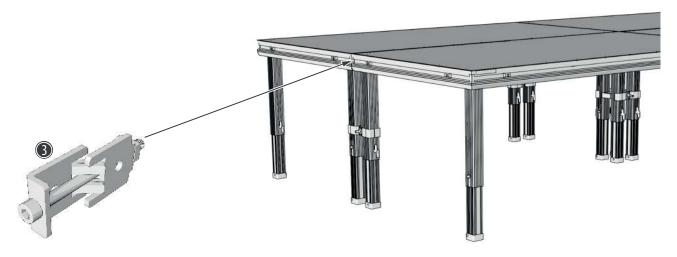
Insert the quick connectors (3) into the profile of the guide rails on the outsides of the stage platforms to be connected and tighten the screws of the quick connectors using an Allen key.
